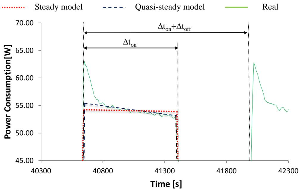
Figure 4. Compressor power consumptions
